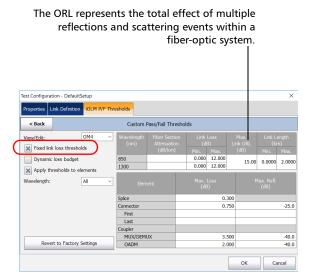
➤ Dynamic: The dynamic loss budget is calculated according to the fiber length and the elements included in the link definition (such as the number of splices, connections, custom elements, as well as splitters).
