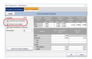
When the fiber type is specified in the link definition (see *Defining the Link for Your Test* on page 92 for details), you can edit thresholds for this fiber type only. If you have selected unspecified as the fiber type, you can specify threshold values for each available fiber type.
