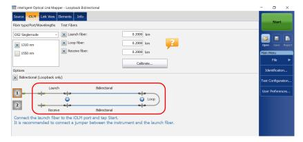
The automatic split of the initial measurement can only be performed if the length of the launch, loop and receive fibers are properly specified in the application. See *Configuring Your iOLM* on page 38 for details.
