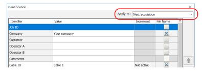
**3.** Select the desired identifiers to include in the file name. You can change the order of appearance of the highlighted component with the up and down arrow buttons.
