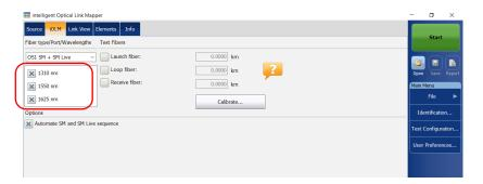
**4.** To enable the automated acquisition sequence, select the **Automate SM and SM Live sequence** check box.
