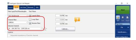
**4.** Specify if launch, receive, and loop fibers are connected to the link under test. See *Launch*, *Receive*, *and Loop Fibers* on page 9 for details.
