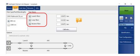
If you want to let the application measure the launch and receive fiber lengths values automatically, go to step 5. You can also specify the launch, receive and loop fiber lengths manually. To do so, go to step 6.
