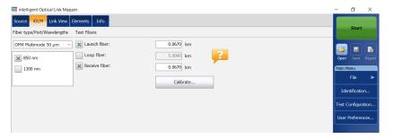
2. If the ICERT software option is activated, select the port to use for your test. The fiber core is also selected at this point; for C fibers, select 50  $\mu$ m, and for D fibers, select 62.5  $\mu$ m.
