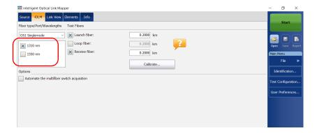
**4.** Specify if launch and receive fibers are connected to the link under test. See *Launch*, *Receive*, *and Loop Fibers* on page 9 for details.
