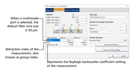
**Note:** The core size cannot be modified for 1550 nm wavelength.
