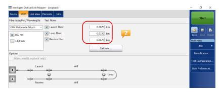
**7.** When the **Loop fiber** checkbox is selected, you can choose to work with the **Bidirectional (Loopback only)** option or not.
