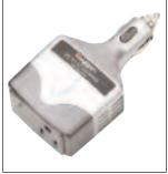
The inverter's output provides a true sine wave rated to deliver 60 watts of ac power continuously or 75 watts of power for 5 minutes. It is also protected with features that will automatically shut off in case of under-voltage, overvoltage, and over-temperature. (Non CE marked.)
