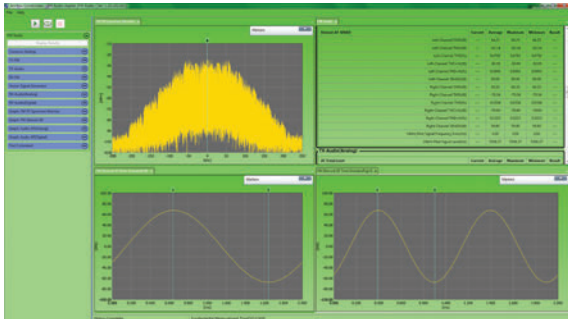
FM Transmitter Test using CombiView
