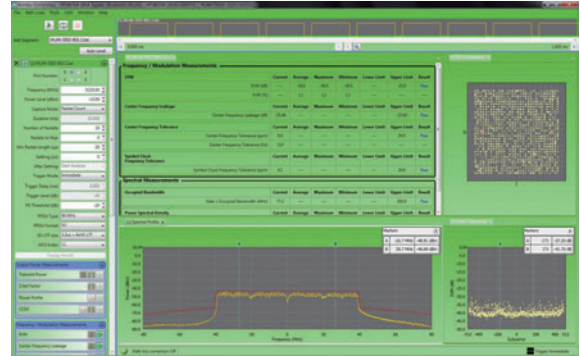
WLAN 11ax TX Measurement using CombiView
