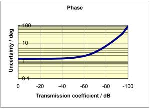
Typical accuracy of transmission magnitude and transmission phase measurements of the R&S $^{\otimes}$ ZVA67 in the frequency range 50 GHz to 67 GHz.
