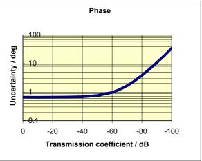
Typical accuracy of transmission magnitude and transmission phase measurements of the R&S $^{\circ}$ ZVA24 in the frequency range 10 MHz to 700 MHz.
