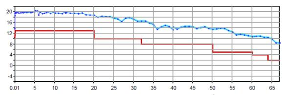
Maximum output power in dBm versus frequency in GHz of the R&S<sup>®</sup>ZVA67.
