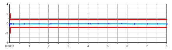
Output power accuracy in dB versus frequency in GHz of the R&S  $^{\!\circ}$  ZVA8.
