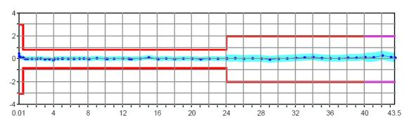
Output power accuracy in dB versus frequency in GHz of the R&S<sup>®</sup>ZVA40.
