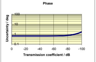
Typical accuracy of transmission magnitude and transmission phase measurements of the R&S®ZVA50 and R&S®ZVA67 in the frequency range 700 MHz to 24 GHz.
