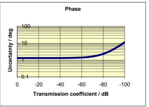
Typical accuracy of transmission magnitude and transmission phase measurements of the R&S®ZVA50 and R&S®ZVA67 in the frequency range 24 GHz to 50 GHz.
