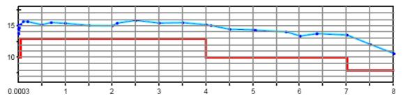
${\it Maximum\ output\ power\ in\ dBm\ versus\ frequency\ in\ GHz\ of\ the\ R\&S^{\&}ZVA8.}$
