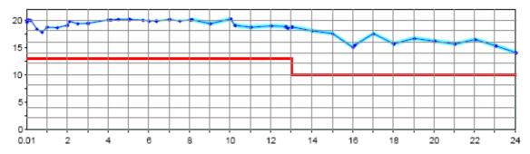
Maximum output power in dBm versus frequency in GHz of the R&S®ZVA24.
