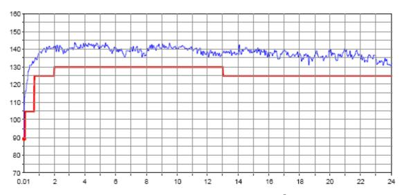
Dynamic range in dB versus frequency in GHz of the R&S®ZVA24.
