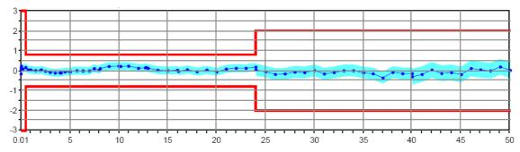
Output power accuracy in dB versus frequency in GHz of the R&S<sup>®</sup>ZVA50.
