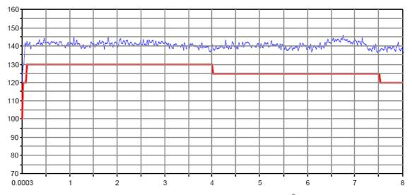
Dynamic range in dB versus frequency in GHz of the R&S®ZVA8.
