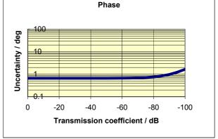
Typical accuracy of transmission magnitude and transmission phase measurements of the R&S®ZVA40 in the frequency range 700 MHz to 24 GHz.
