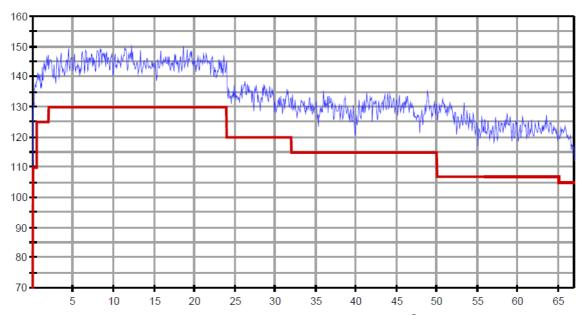
Dynamic range in dB versus frequency in GHz of the R&S®ZVA67.
