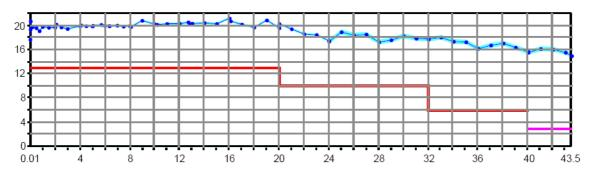
Maximum output power in dBm versus frequency in GHz of the R&S<sup>®</sup>ZVA40.
