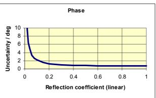
Typical accuracy of reflection magnitude and reflection phase measurements of the R&S®ZVA8 in the frequency range 1 MHz to 8 GHz, of the R&S®ZVA24 in the frequency range 50 MHz to 24 GHz, of the R&S®ZVA40 in the frequency range 50 MHz to 40 GHz, of the R&S®ZVA50 in the frequency range 50 MHz to 50 GHz and of the R&S®ZVA67 in the frequency range 50 MHz to 67 GHz.
