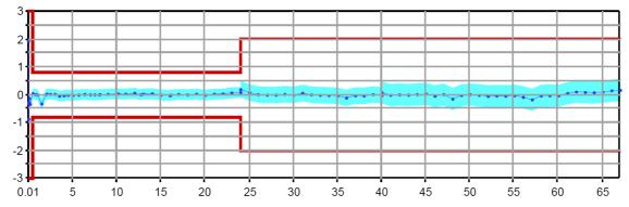
Output power accuracy in dB versus frequency in GHz of the R&S $^{\otimes}$ ZVA67.
