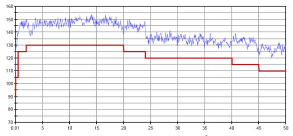
Dynamic range in dB versus frequency in GHz of the R&S®ZVA50.
