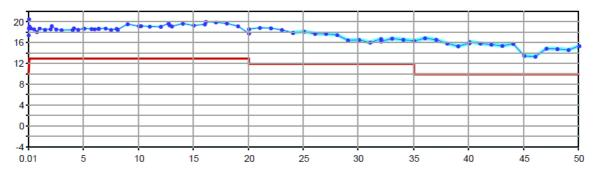
Maximum output power in dBm versus frequency in GHz of the R&S®ZVA50.
