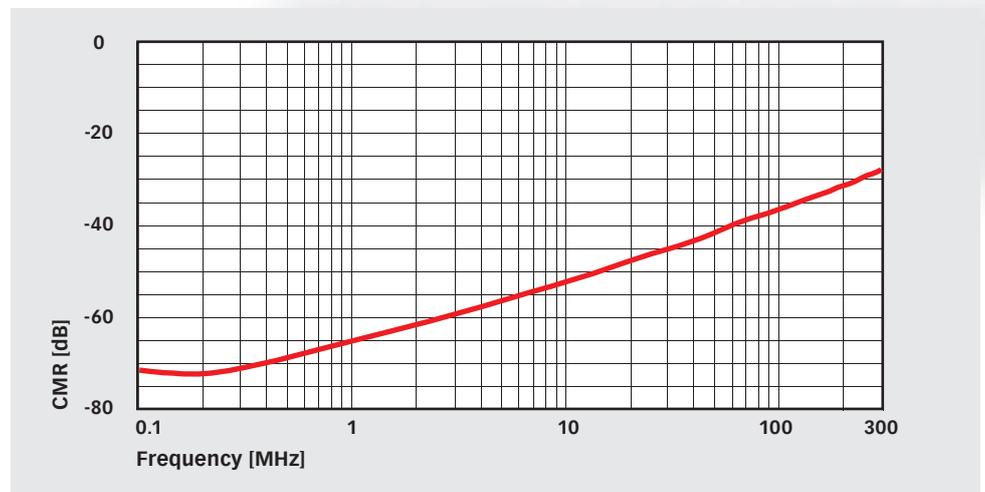
Example for measuring the transmission of the ISN
