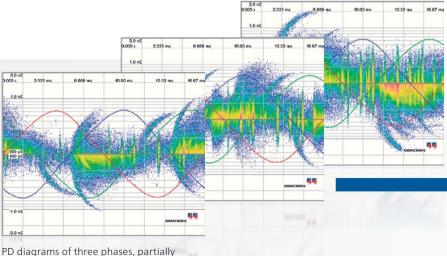
PD diagrams of three phases, partially superimposed or with interference signals
