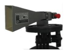
Frequency Range: 18 GHz - 26.5 GHz Antenna Factor (1 Meter) 36.7 to 37.1 Gain (dBi) 18.6 to 21.6 Maximum Continuous Power: 50 Watts Max Radiated Field: 200 V/m Beamwidth 15° Impedance: 50  $\Omega$  Connector: WR-42 to SMA female Mounting Base:  $\frac{1}{4}$  - 20 Thread, female
