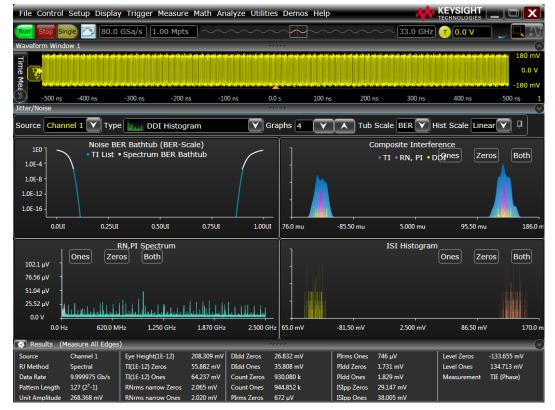
Discover signal anomalies in the amplitude noise domain of the waveform
