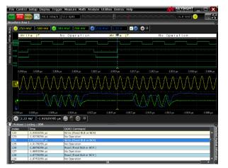
DDR3 protocol decode and write command trigger.
