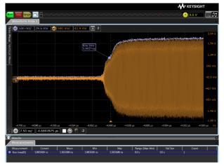
Envelope detection of signal burst.
