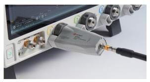
N7010A active termination adapter provides a low noise single-ended cabled measurement solution with 50  $\Omega$  voltage termination (V<sub>TERM</sub>) up to 30 GHz bandwidth.
