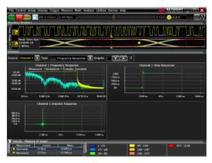
InfiniiSim renders the waveform through hardware acceleration.
