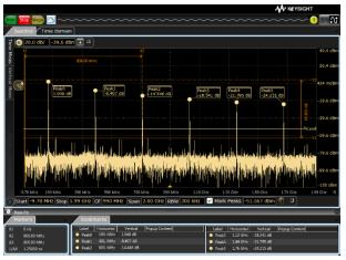
Peak readouts in the FFT plot.
