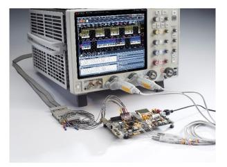
DDR3 test setup with mixed signal oscilloscope.
