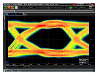
DDR3 write data burst eye-diagram analysis.
