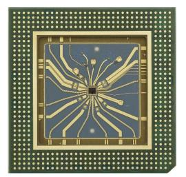
Keysight uses Indium Phosphide process to produce a 12 ps edge step response, ideal for characterizing cable and probe frequency response.
