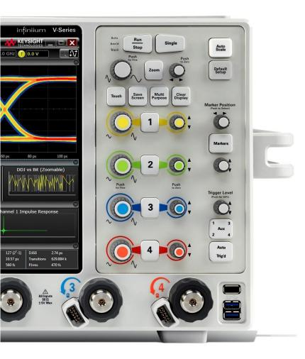
Threaded 3.5 mm RF connectors with convenient torque mechanism ensures the most reliable signal integrity and consistent 8 in. Ibs. connection. The AutoProbe II interface provides a robust interface for the InfiniiMax III and III+ probing system. New industrial design and front panel layout that enhances user experience and operation of the oscilloscope.
