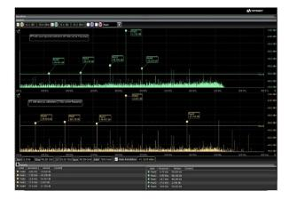
Improved calibration increases the spurious free dynamic range by up to 15 dBc.
