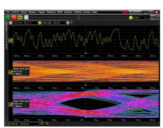
Serial data equalization opens the closed eye using CTLE and DFE methods.
