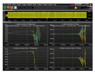
The magnitude and phase response of a cable corrected using PrecisionProbe.
