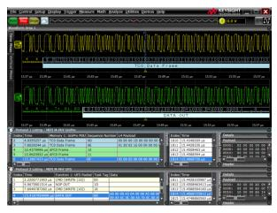
Packet decode and CRC verification through the oscilloscope MIPI UniPro and UFS protocol decoders.
