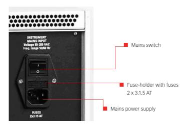
To insert a fuse, pull the fuse-holder out of the connector, insert 2 fuse cartridges 2 x 3.15 AT (slow blow) into the holder and put the holder back.
