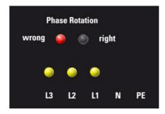
Not all EUT power lines provide power and the phase rotation is wrong too. All phase of the EUT in power need to be checked and re-plugged.
