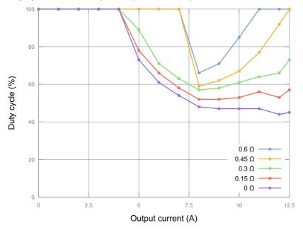
Duty cycle at + 25 °C (+ 77 °F) ambient temperature
