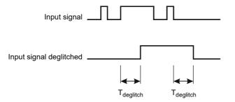
Figure 2-2: Signal curve, deglitching input signals
