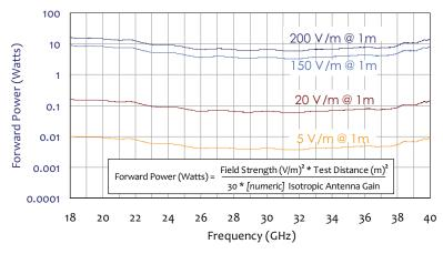
FIGURE 15 - Power requirements for various fields strengths/distances
