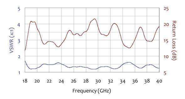
FIGURE 18 - Typical VSWR/Return Loss at Coaxial Antenna Port
