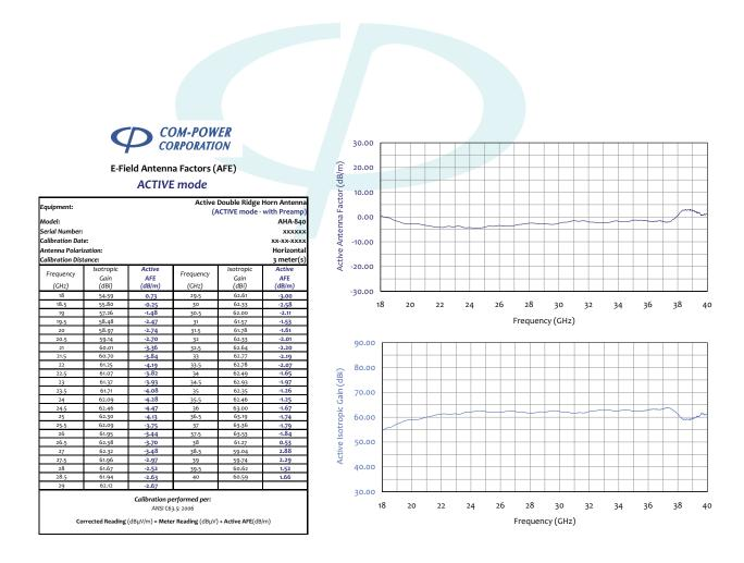
FIGURE 16 - Typical ACTIVE Antenna Factors/Gain Values
