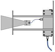
By calibrating the ACTIVE mode as a system, rather than calibrating the antenna, cable and preamplifier individually, any mismatches that occur between components are accounted for in the antenna factor. This system level approach yields much more accurate results (factors) than those achieved through individual calibration of the components.
