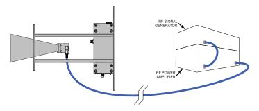
FIGURE 13 - Typical test setup for ACTIVE-Tx Configuration
