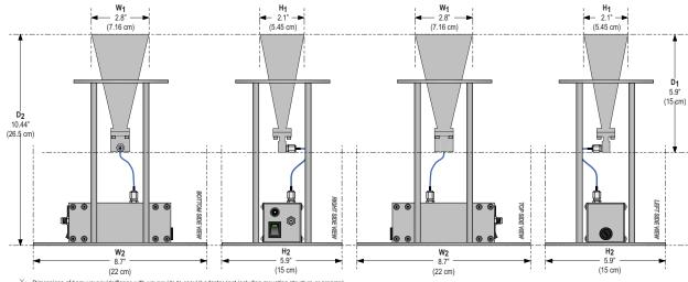
X<sub>1</sub> - Dimensions of horn waveguide/flange with waveguide to coaxial adapter (not including mounting structure or preamp)
