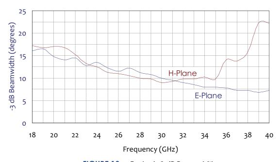
FIGURE 19 - Typical -3 dB Beamwidth
