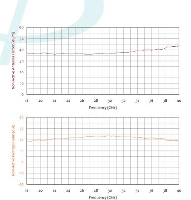
FIGURE 17 - Typical NON-ACTIVE Antenna Factors/Gain Values
