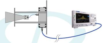
FIGURE 7 - Typical setup for ACTIVE-Rx (Std) mode
