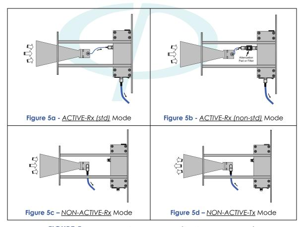
FIGURE 5 - Antenna Configurations (Modes of Operation)
