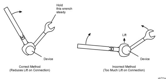
2. Hold the torque wrench lightly, at the end of the handle only (beyond the groove). See Figure 3-7.
