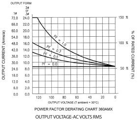
Short term overloads to 150% are permitted. Operating time before thermal shutdown or circuit breaker trip varies from seconds to several minutes depending upon line and temperature conditions.
