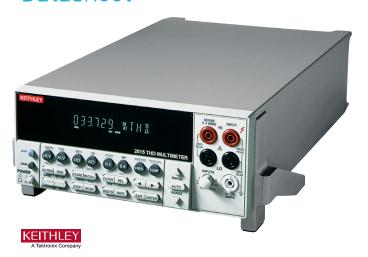
The 2015-P Audio Analyzing Digital Multimeter and the 2015 Total Harmonic Distortion Multimeter combine audio band quality measurements and analysis with a full-function 6½-digit DMM. Test engineers can make a broad range of voltage, resistance, current, frequency, and distortion measurements, all with the same compact, half-rack measurement instrument. The 2015-P offers additional processing capacity for frequency spectrum analysis.
