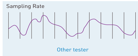
General charger/discharger sampling rate
